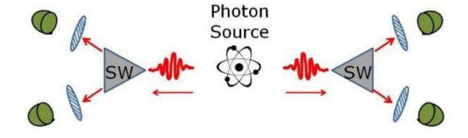
Schematic of the third Aspect experiment testing quantum non-locality. Entangled photons from the source are sent to two fast switches that direct them to polarizing detectors. The switches change settings very rapidly, effectively changing the detector settings for the experiment while the photons are in flight. (CHAD ORZEL)
