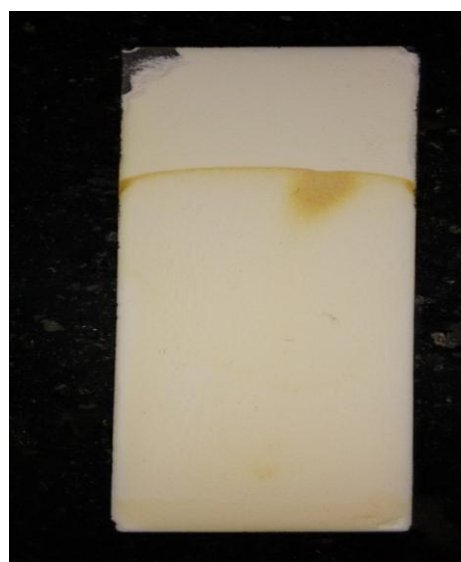
Fig. 3b: TLC plate with single spot after the separation using chloroform as a solvent system.
