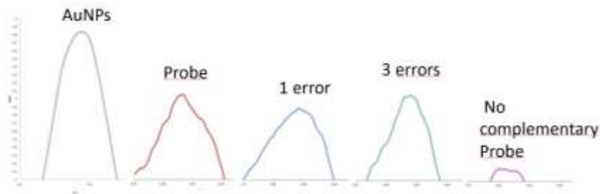
Figura 8. Voltamperograms DPV of the genosensor with the complementary probe, an error, 3 errors and not complementary for S. Typhi
