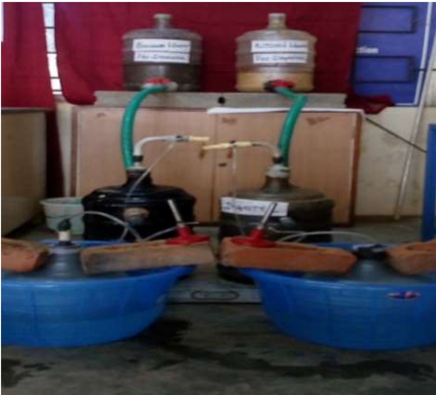
Fig.2. BIOGAS PRODUCTION UNIT
