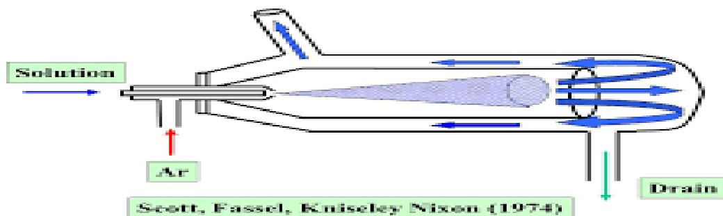
**Fig10-Scott double pass spray chamber**
