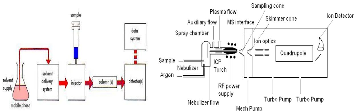
Fig7-interface 1 from column to nebulizer
