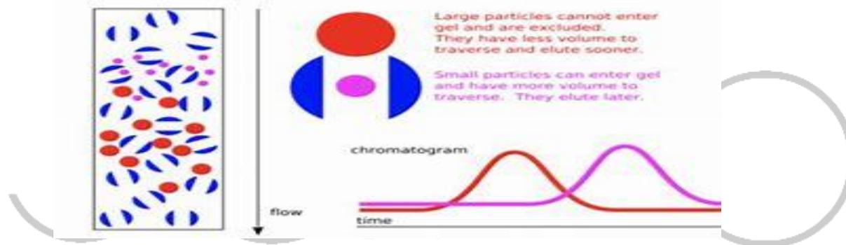
Fig5-particle size in the stationary phase
