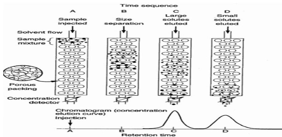
Fig2-mechanism of size exclusion chromatography
