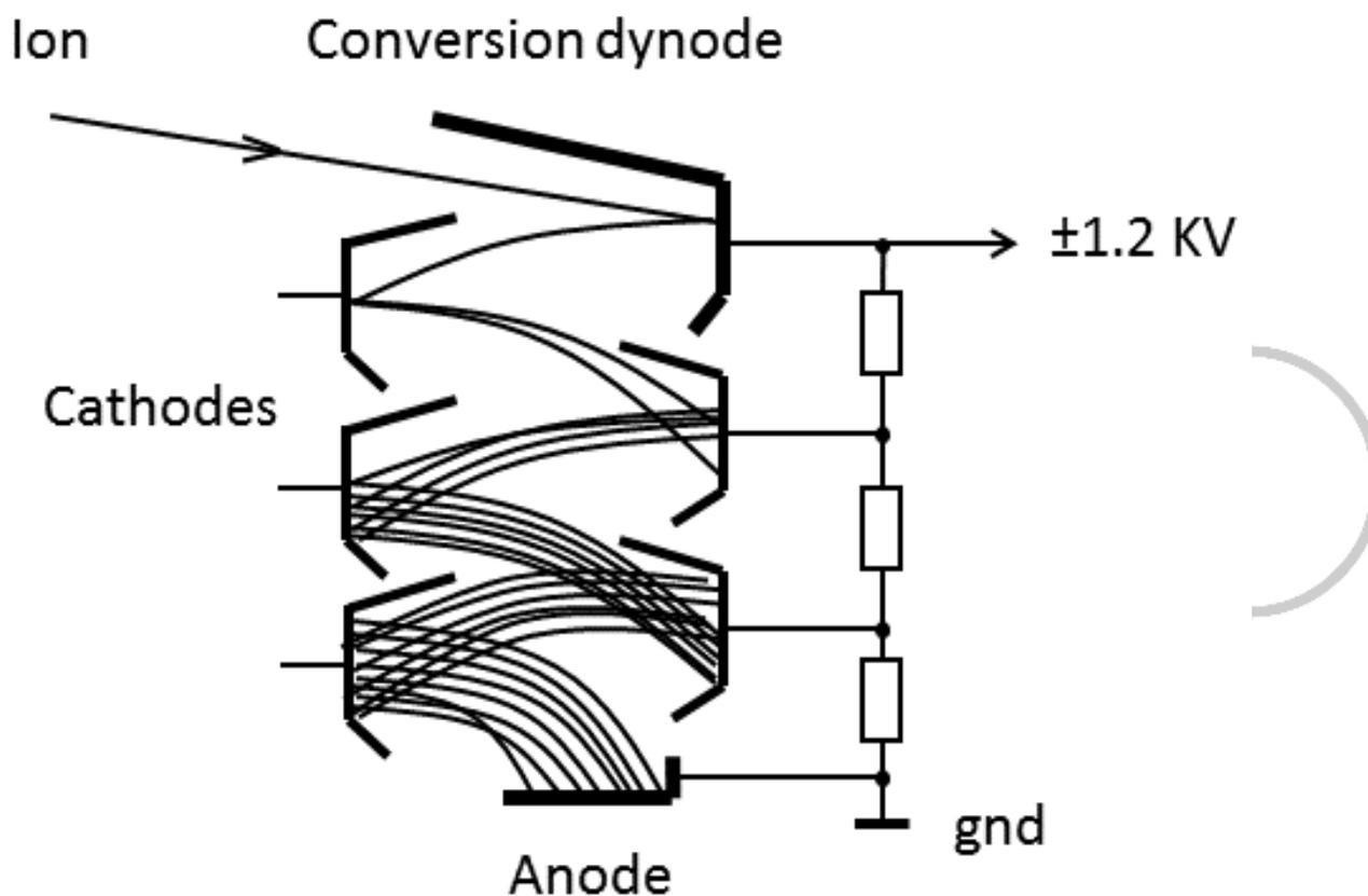
Fig14-electron multiplier tube
